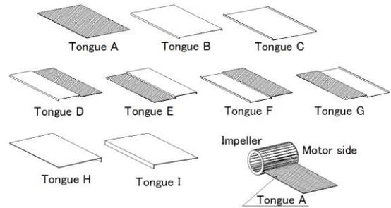
Fig. 3 Nine configurations of the tongues in experiment
