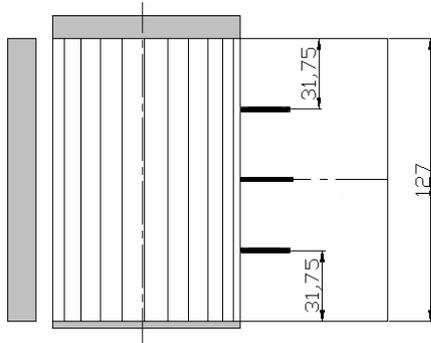
**Fig. 10** Mounting points of sensors for measuring sound, pressure and velocity
