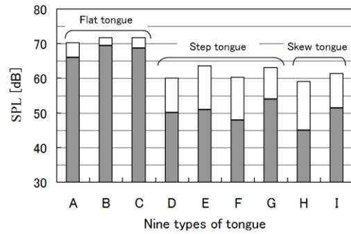
**Fig. 7 Overall noise level and rotation noise level for 9 types of tongue**
