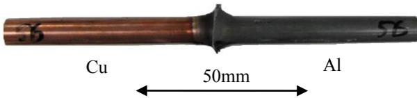
Fig.3 Appearance of the welded joint
