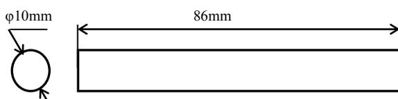
**Fig. 2 Shape and dimension of the specimen**
