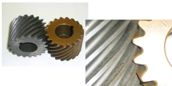
Fig. 2 View of crossed helical gears
