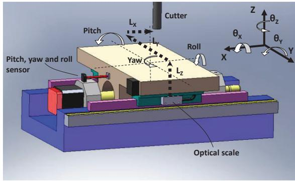
Fig. 7 Machine tool with embedded sensor module
