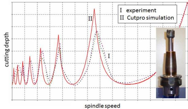
Fig. 5 High speed cutting of AlMg4,5Mn (Heller MCI 16.2, PCD face milling cutter Ø24mm, z = 4)
