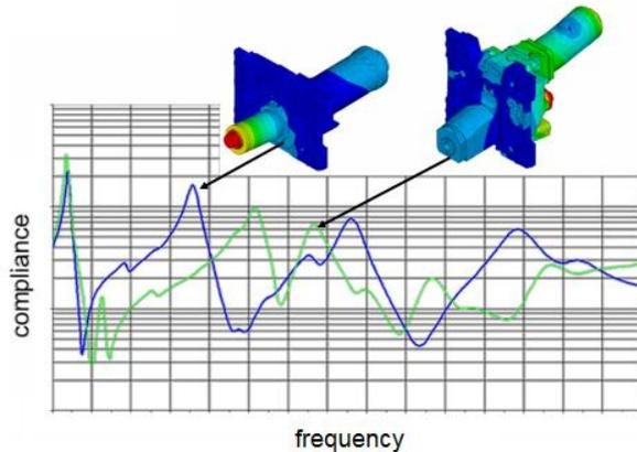
**Fig. 3 Compliance responses of cutting units**
