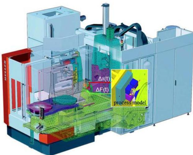
**Fig. 6** FE simulation of Heller H5000 with integrated cutting process for the prediction of stability charts
