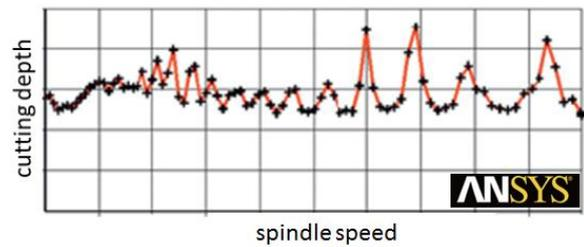
**Fig. 7** Stability chart gained from FE simulation with integrated cutting process
