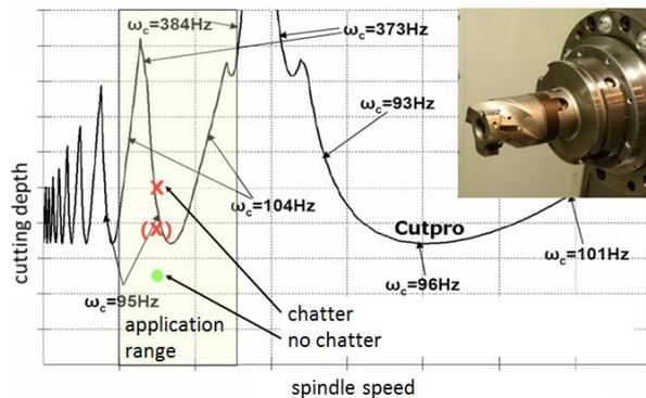
Fig. 4 Predicted stability chart on the basis of compliance responses from FE simulation
