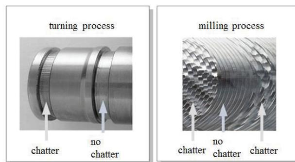
Fig. 1 Turning and milling workpiece surface quality with and without regenerative chatter
