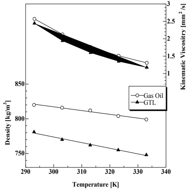
Fig. 1 Density and kinematic viscosity
