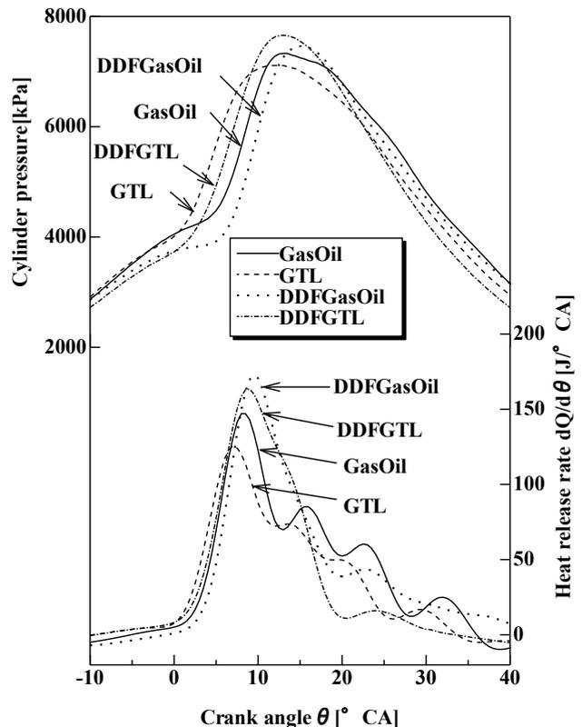
Fig. 4 Cylinder pressure and heat release rate at the highest load
