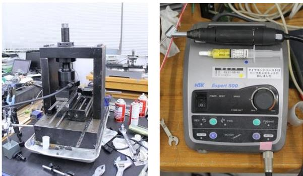
**Fig. 4 The endurance test machine (left) and polishing equipment for surface finish (right)**
