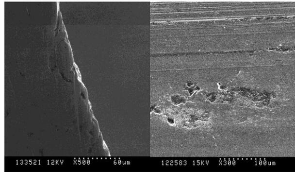
a) Rolling contact surface    b) Severely damaged rail guide
