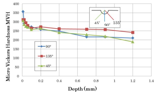
**Fig.9** Changes of Micro Vickers hardness of 18-8 stainless steel vicinity of the groove in radial direction after roller burnishing
