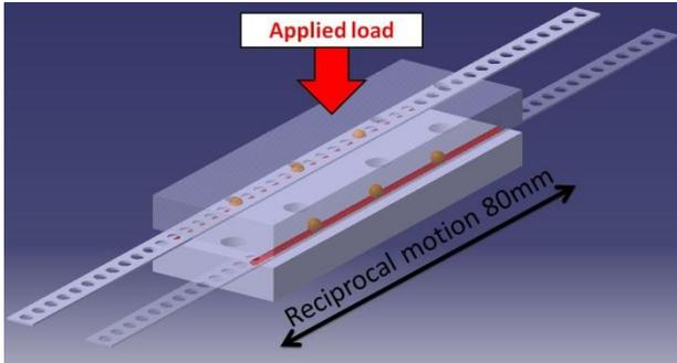
**Fig. 3 Geometry of specimen plate and balls with retainer**
