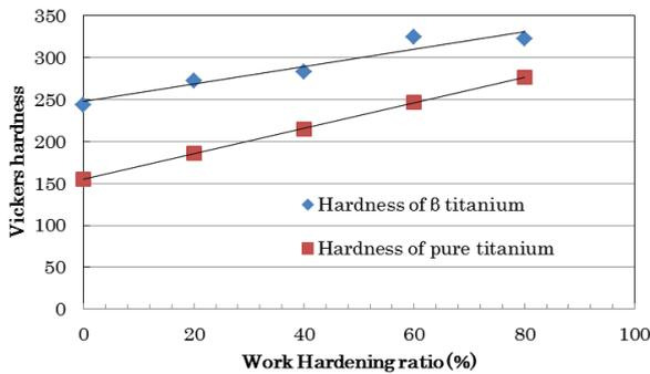
**Fig.10 Changes of Vickers hardness of titanium by work hardening**
