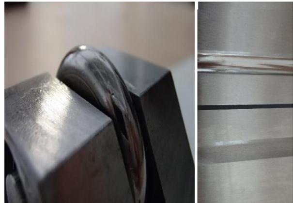
**Fig. 5 The work hardening roller (burnishing roller) (left) and before (lower right) and after (upper right) of work hardened specimen**
