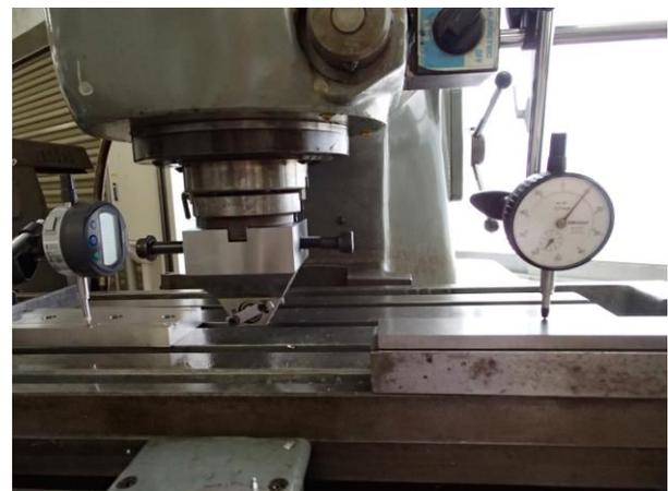
**Fig. 6 The milling machine assembled with work hardening tooling (burnishing roller)**
