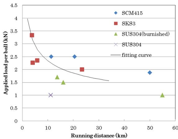
**Fig.11 Life of rolling distance for miscellaneous materials**
