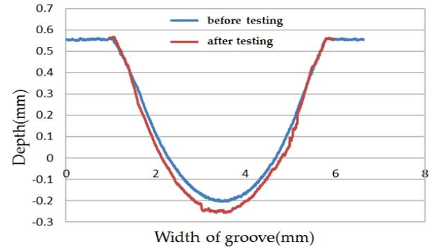
**Fig. 8** Changes of cross-sectional shape of the groove for as received SUS304 after testing
