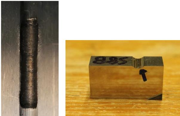
**Fig. 13** Damages on the groove(left) and cross-cut of the groove(right)
