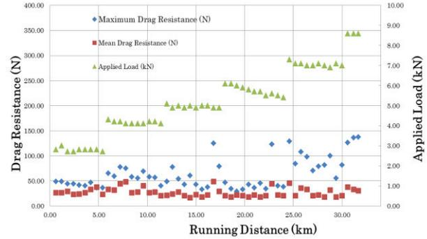
**Fig.7** Changes of drag force in endurance test for SUS304
