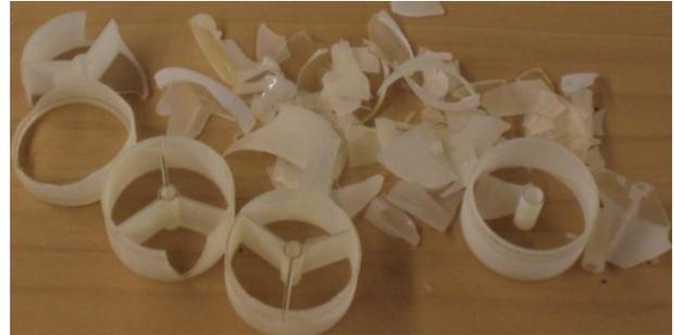
**Fig. 6 Two more or less intact half cylinder and lots of broken pieces**
