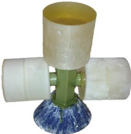
**Fig. 2 Mounted cluster with hollow cylinder with pillar, solid cylinder, and hollow cylinder having 3 ribs (f.l.t.r.)**
