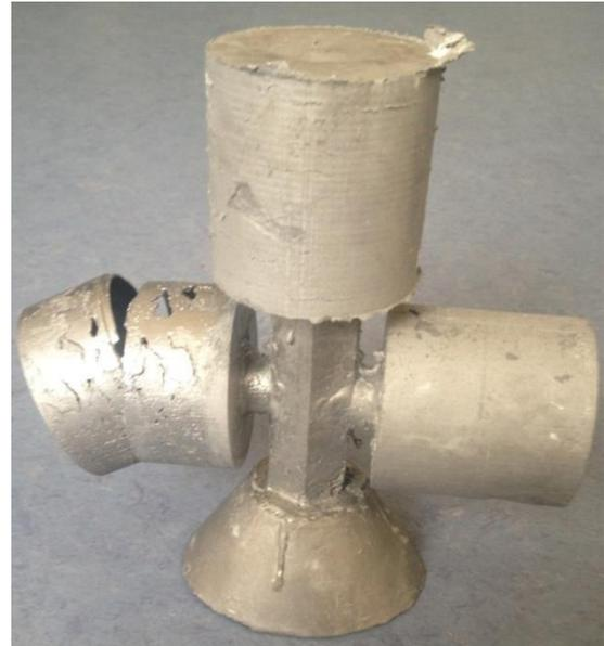
**Fig. 3 Intact cylinder and defect casting**
