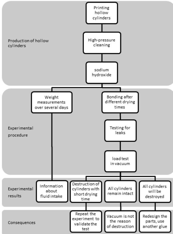
**Fig. 4 Process of the experimental procedure and the expected results with the appropriate consequences**
