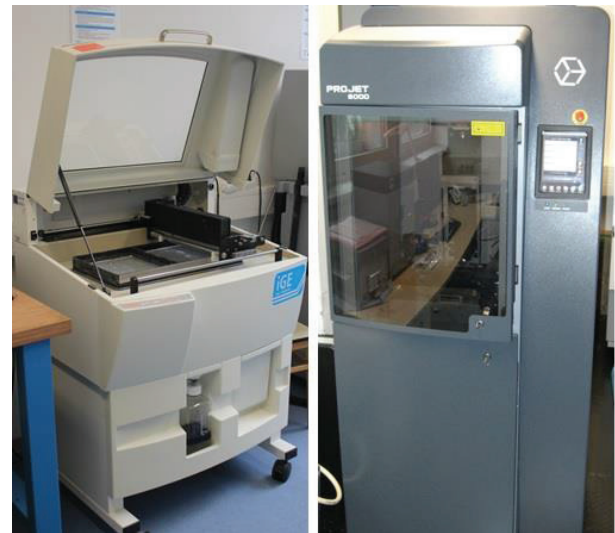
(a) 3D printer ZPrinter® 310 (b) Stereolithographic system ProJet® 6000
